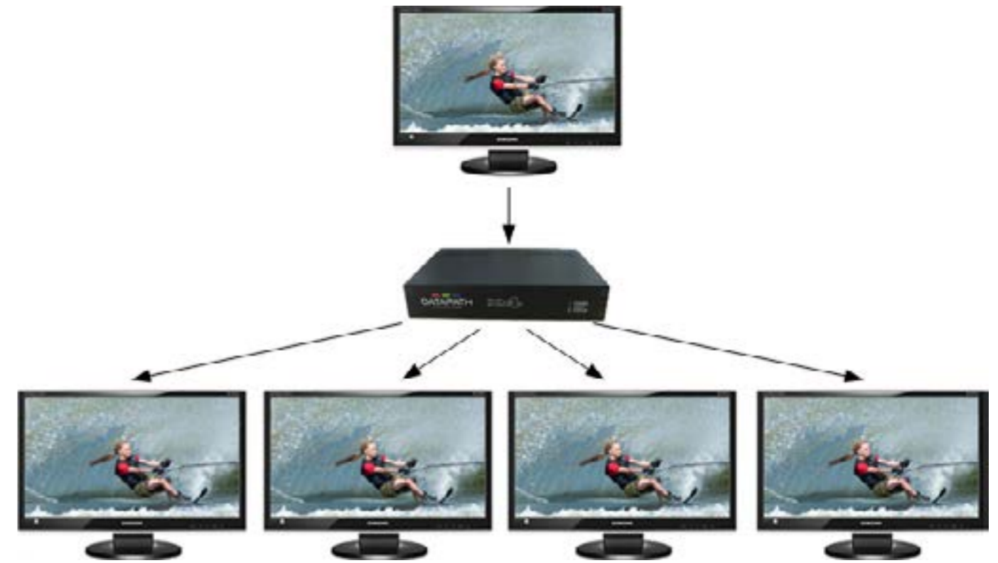
Duplicate the input signal x 4 and displays each duplicate on separate screens
